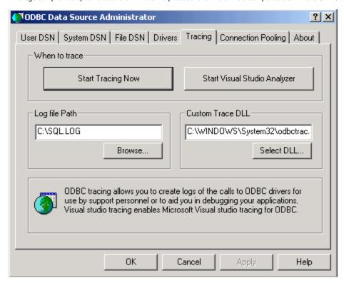
The trace slows down the ODBC connection, but the output to the log can be useful.
