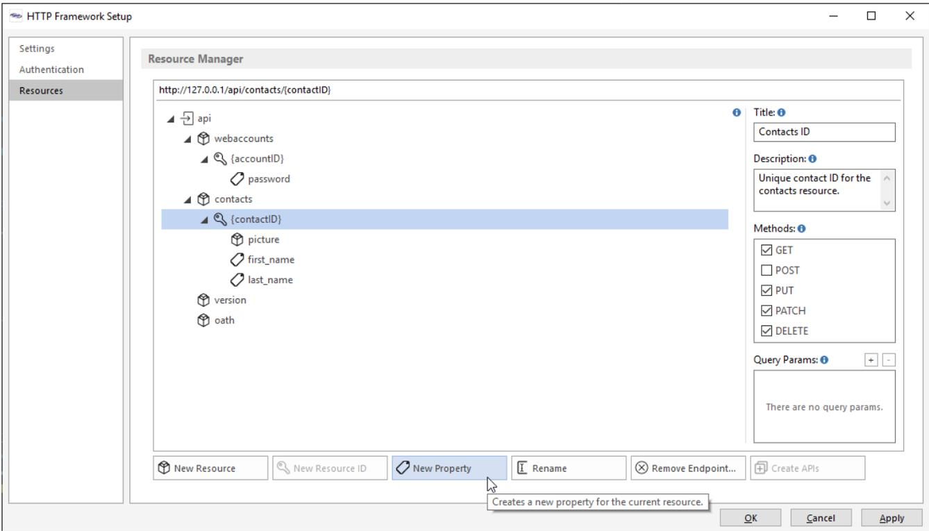
Resource definition data is managed using the [HTTP\\_Resource\\_Manager\\_Services](#) module. Note: [SRP\\_HTTP\\_FRAMEWORK\\_RESOURCES](#) is the default configuration row for all applications. Each local application will copy this and maintain a local version using the format [SRP\\_HTTP\\_FRAMEWORK\\_RESOURCE S\\*<AppID>](#).
