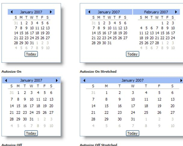
**When Autosize is disabled, all months expand to fit the control. When Autosize is enabled, the months maintain a balanced margin.**
